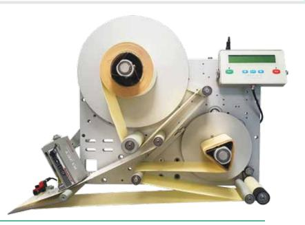
The AL150 TIJ modular labeler is a labeling system of the 150 series.
