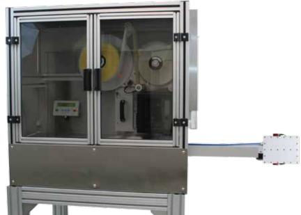
**AP190 RT** is an automatic print & apply system, suitable for A5 labels application on multiple sides of a pallet, according to the international logistic identification standards. The applicator pad of **AP190 RT** is mounted on a programmable axis, turnable ±90°, allowing both landscape and portrait label orientation without further regulations.
