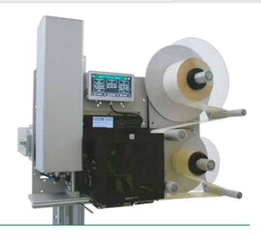
The AP150 pneumatic linear applicator is a print & apply system of the 150 series.
